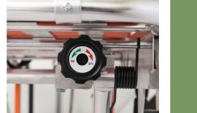
**Safety Lock** The safety lock is locked when transporting a patient, and unlocked when getting on an ambulance.
